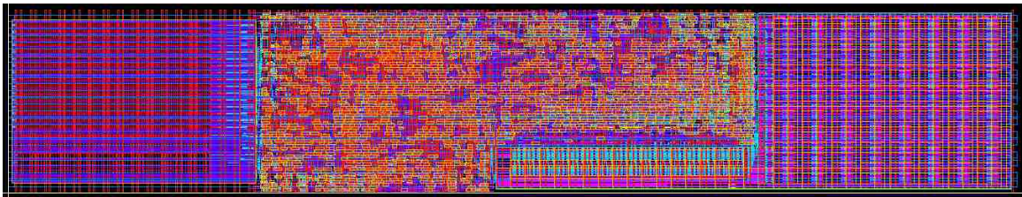
Figure 2: JFP layout in a 65nm technology with dimensions of 830µm x 150µm.
